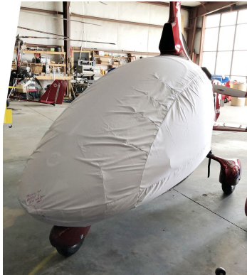
Cavalon Gyrocopter Bubble Cover, test fit cover
