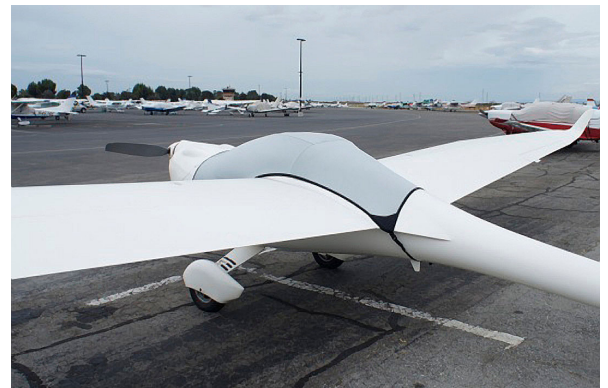
Lambada Canopy/Engine Cover and Wing Covers
