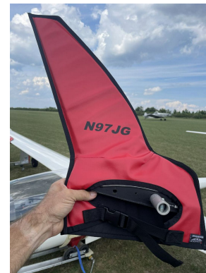
Schempp-Hirth Ventus-2B winglet/wingtip pads
