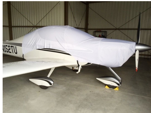
Tecnam Astore Canopy/Engine Cover, test fit cover
