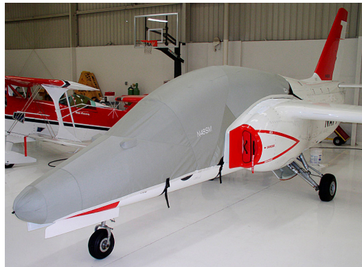
S-211 Canopy/Nose Cover & Engine Plugs
