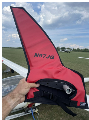
Schempp-Hirth Ventus-2B winglet/wingtip pads
