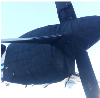
ATR-72-202 Insulated Engine & Prop Hub Covers
