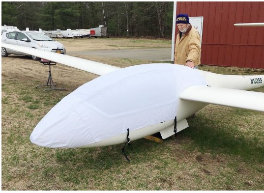
Grob 102 Astir CS Canopy/Nose Cover (test fit)
