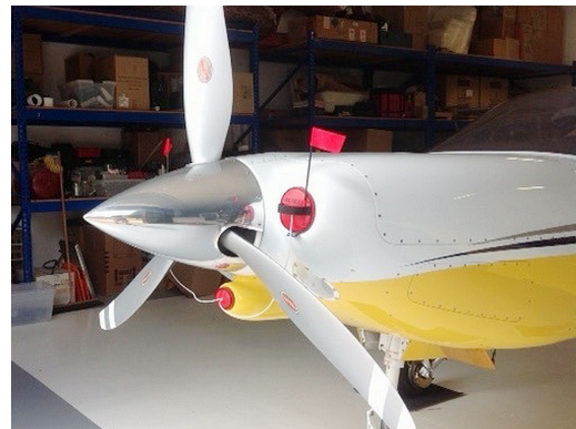
Swearingen SX300 Engine Inlet Plugs
