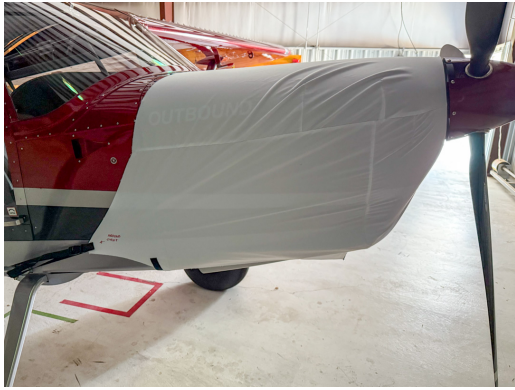
Rans S-21 Engine Cover, test fit cover
