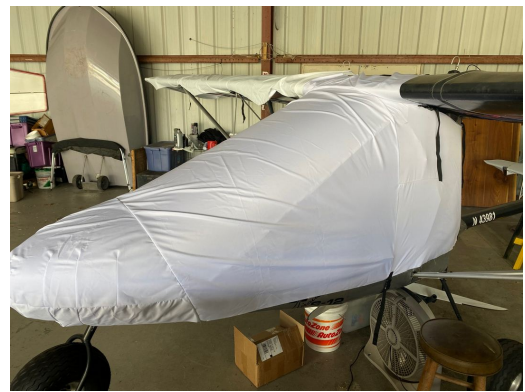
Rans S-12 Canopy/Nose Cover, test fit
