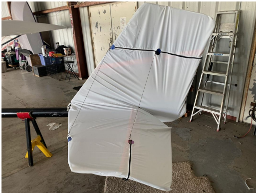
Rans S-12 Empennage Cover, test fit
