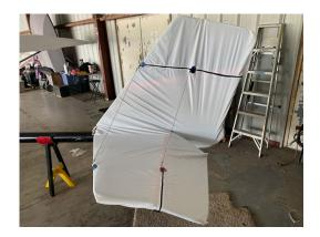
Rans S-12 Empennage Cover, test fit
