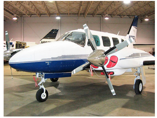
Piper Navajo PA31 Engine Inlet Plugs (Panther Conversion)
