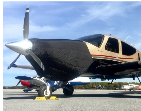
Rockwell Aero Commander Insulated Engine Cover
