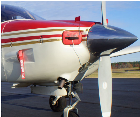
Rockwell Aero Commander 112, 114 Engine Inlet Plugs (112 Model)
