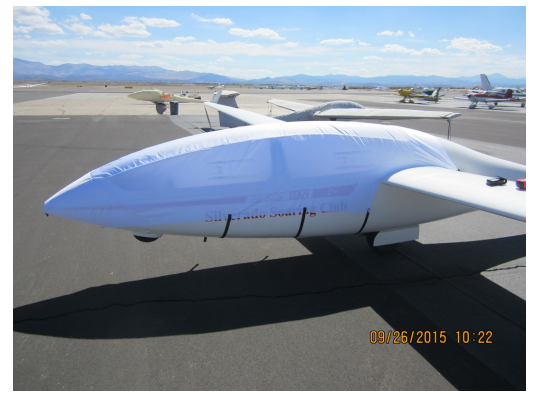
DG-505 Canopy/Nose Cover (test fit cover)
