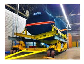
PW JT9D Series Off-Link Engine Transport Cover, Fully Enclosed, P/N: PW-120
