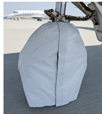
CJ1 Nose Gear Tire Cover, test fit
