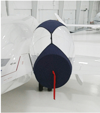
Challenger 300 Intake/Exhaust Cover Set, 3-strap type Pitot, AOA, Ice Detector Covers (PRE-200) and Engine Inlet Plugs (PRE-100)
