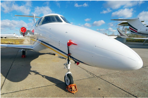
Challenger 300 Intake/Exhaust Cover Set, 3-strap type Pitot, AOA, Ice Detector Covers (PRE-200) and Engine Inlet Plugs (PRE-100)
