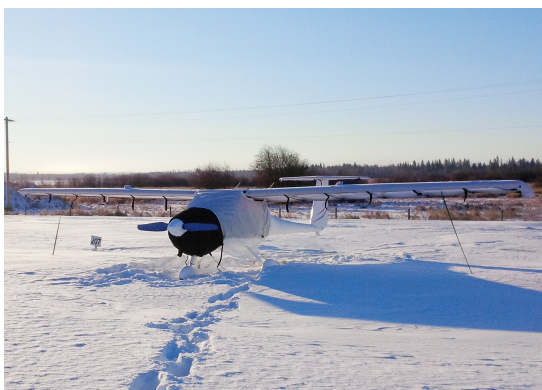
Pipistrel Canopy, Wings, Tail & Insulated Engine Covers
