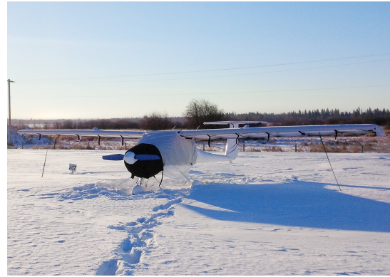
Pipistrel Canopy, Wings, Tail & Insulated Engine Covers
