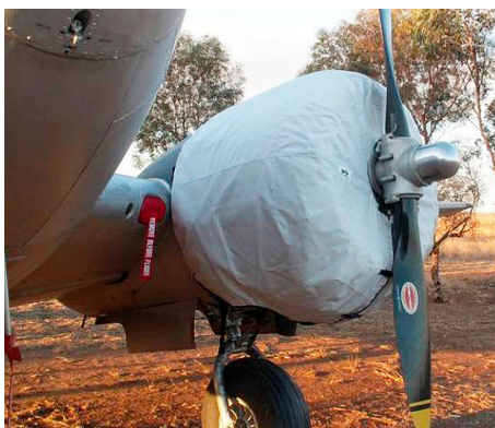
Beech D-18 Engine Covers, Center Section Oil Cooler Inlet Plugs, and Pitot Covers
