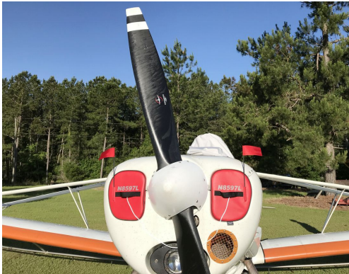
Piper Pawnee PA-25 Engine Inlet Plugs
