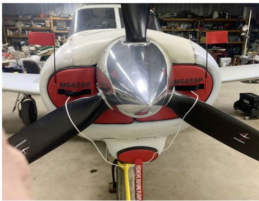
Piper PA-24 Comanche Engine Inlet Plugs
