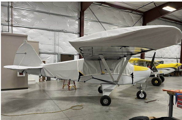
Piper PA-22-108 Canopy Cover, Over Top type
