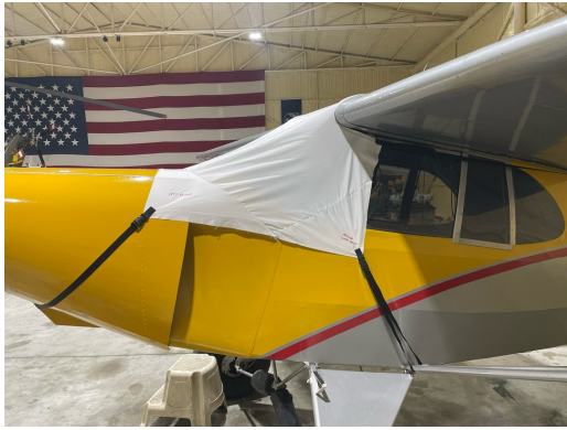
Piper J5A Windshield/Skylight Cover, test fit
