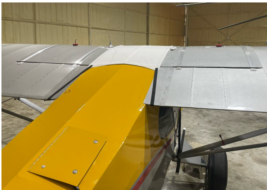
Piper J5A Windshield/Skylight Cover, test fit
