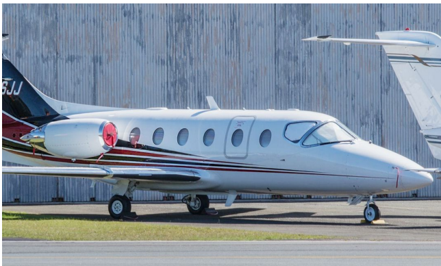
Beechjet Engine Plugs and Cockpit Heatshields
