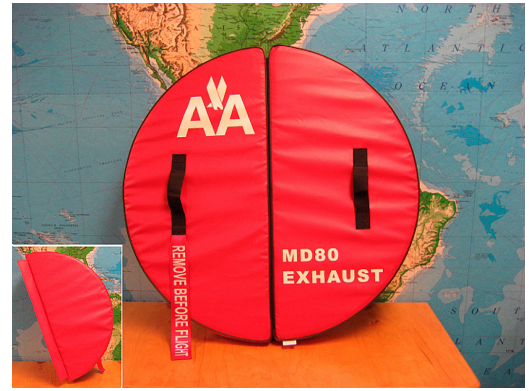
MD-80 Exhaust Plug, folding type
