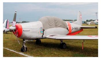
Pilatus PC-9 Canopy Cover, Prop Tie-Down, Engine Plug, Pitot Cover
