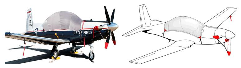
Texan II T6A Canopy Cover, Engine Inlet Plug, Prop Tie/Exhaust Pilatus PC-9 Canopy Cover, Prop Tie-Down, Engine Plug, Pitot Cover, Pitot Cover
