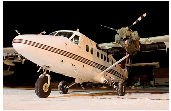
De Havilland Twin Otter Insulated Engine & Insulated Propellor/Spinner Covers Twin Otter Wing, Horiz. Stab & Engine Covers
