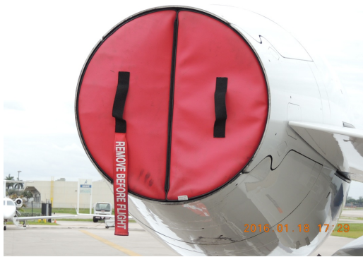
Embraer Legacy 500 Engine Exhaust Plug, folding type
