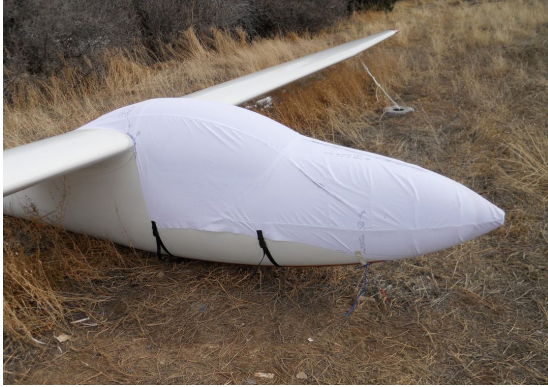
Laister LP-49 Canopy/Nose Cover, test fit cover
