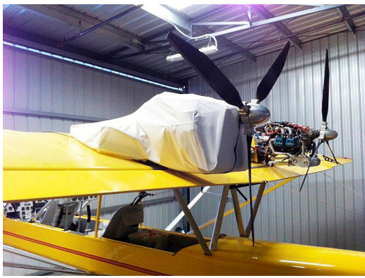
Lockwood AirCam Engine Cover (test fit cover)
