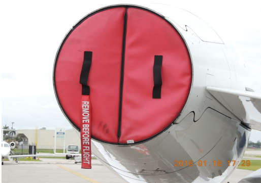
Embraer Legacy 500 Engine Exhaust Plug, folding type
