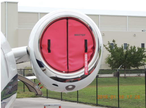
Embraer Legacy 500 Engine Inlet Plug, folding type
