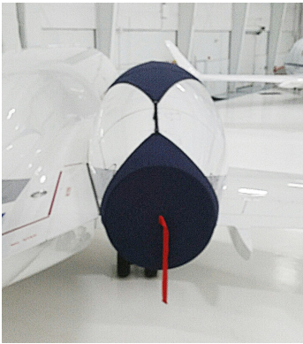
Challenger 300 Intake/Exhaust Cover Set, 3-strap type
