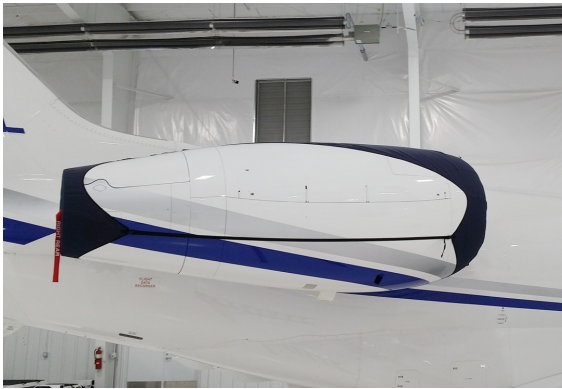
Challenger 300 Intake/Exhaust Cover Set, 3-strap type
