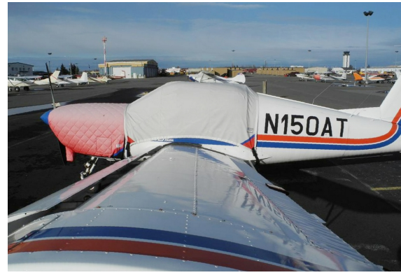
Kolibler 150A Canopy Cover, Insulated Engine Cover
