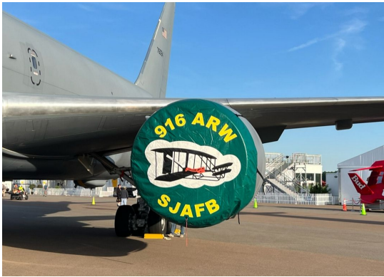
Boeing KC-135 Intake Covers, soft type, CFM56 engines
