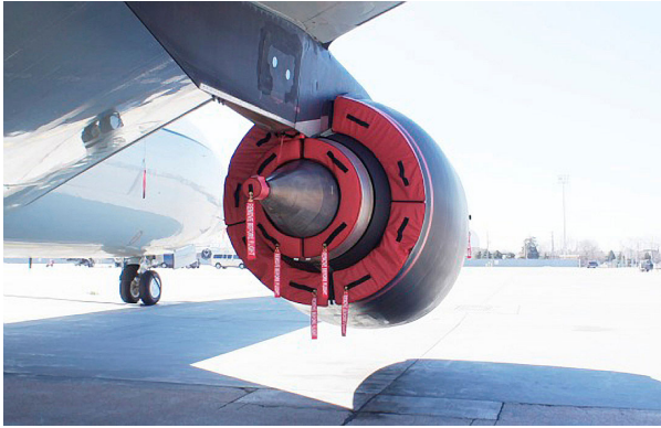
RC-135W Bypass Vent and Exhaust Plugs
