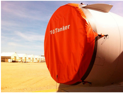
DC-10-30 Intake Cover (CF650C2 Engine)
