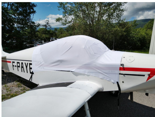
Jodel D113V Canopy Cover, test fit cover
