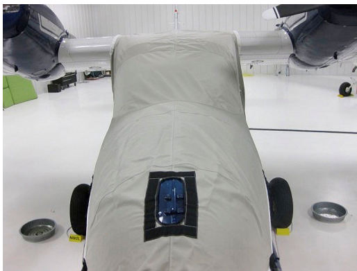
Grumman Widgeon Cockpit/Nose Cover, tie-down cleat detail
