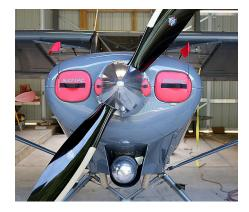
Piper PA-18 Super Cub Engine Inlet Plugs
