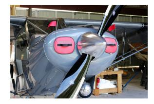
Piper PA-18 Super Cub Engine Inlet Plugs
