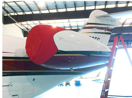
Canadair Challenger 300 Intake/Exhaust Covers, 3-Strap Type
