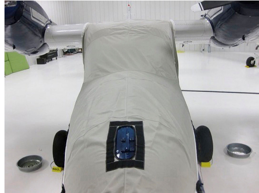
Grumman Widgeon Cockpit/Nose Cover, tie-down cleat detail
