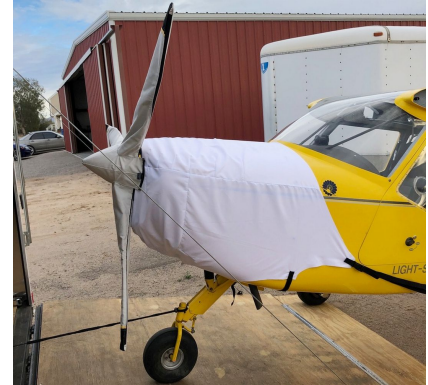
FK-9 Engine Cover, test fit cover
