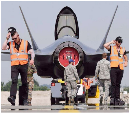
Lockheed Martin F-35 Exhaust Plug, non-folding type
