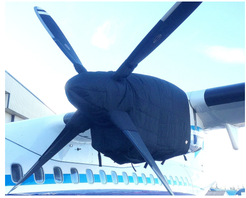
ATR-72-202 Insulated Engine & Prop Hub Covers
