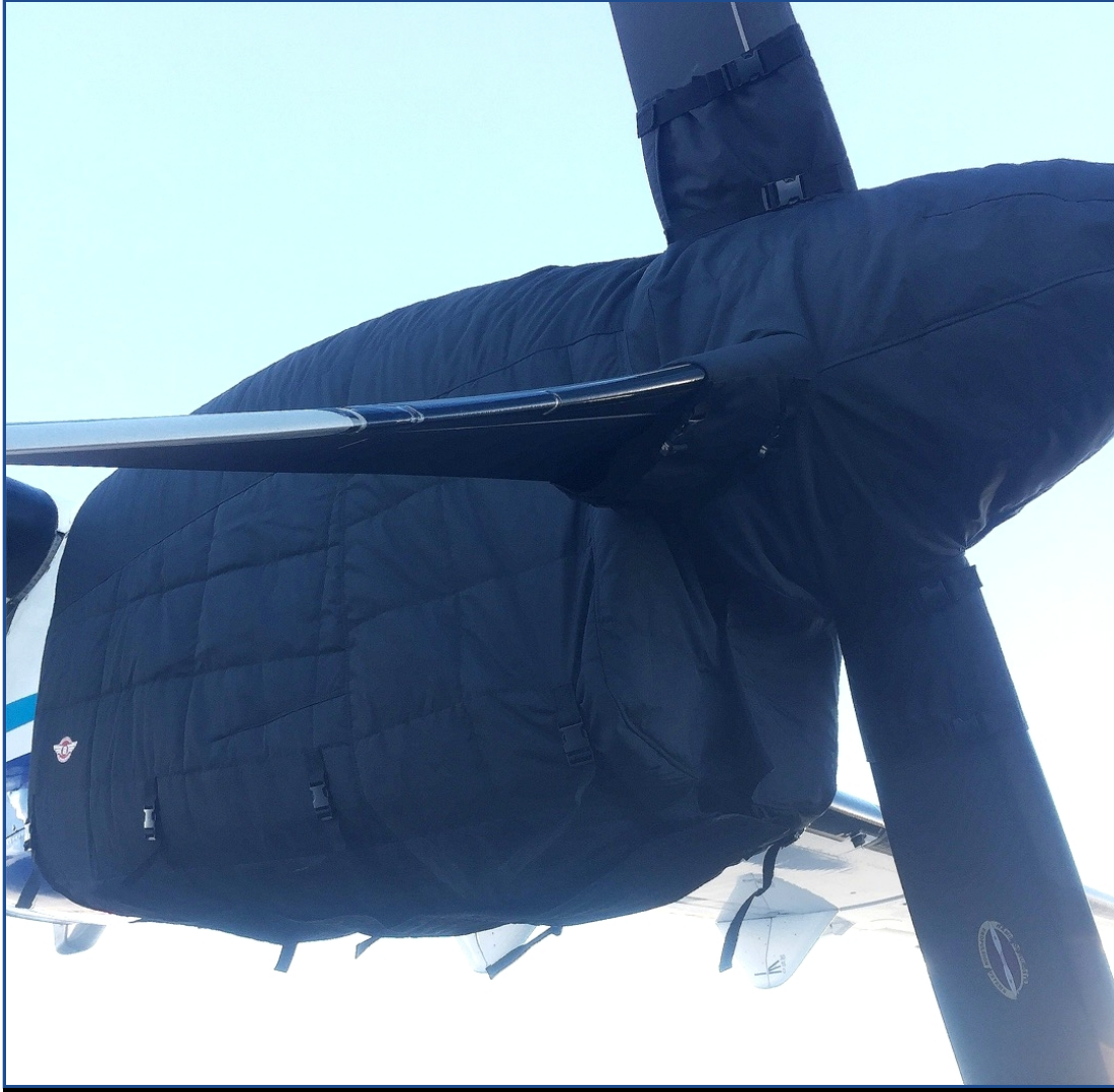
ATR-72-202 Insulated Engine & Prop Hub Covers
