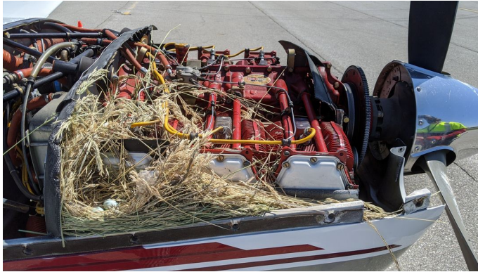
ENGINE PLUGS PREVENT BIRD NEST FOD. Piper Saratoga Engine Cowling Covers, Plugs & HeatShields for the Extra 400 Bird's Nest
