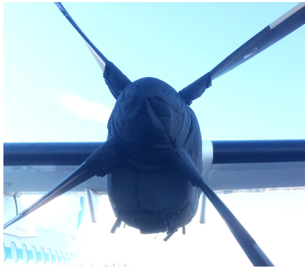
ATR-72-202 Insulated Engine & Prop Hub Covers
