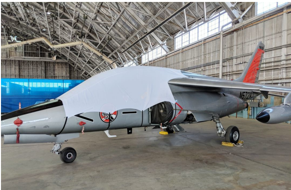
Dornier Alpha Jet Canopy Cover, test fit cover
