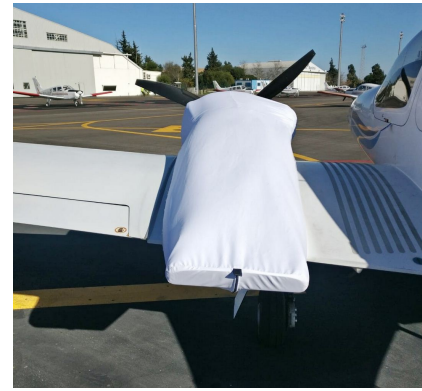
DA42 MPP Guardian (DA42-NG) Engine Cover, test fit cover
