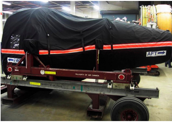
CFM-56-5A/5B Off-link Engine Shipper/Transport cover, w/ Exhaust Cone, fully enclosed
