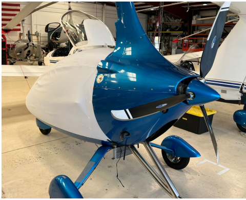
Autogyro Calidus Canopy/Nose Cover, test fit cover
