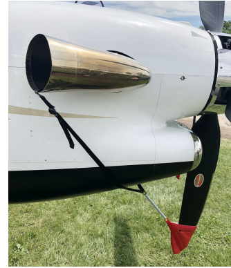
Beech C90A Prop Tie-Down
