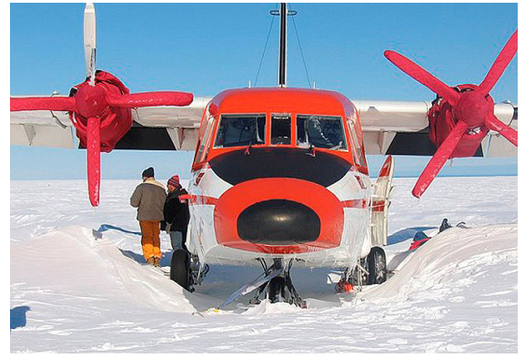
Casa 212 Insulated Engine & Propellor/Spinner Covers
