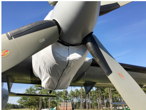
Casa 212 Engine Cover, test fit cover
